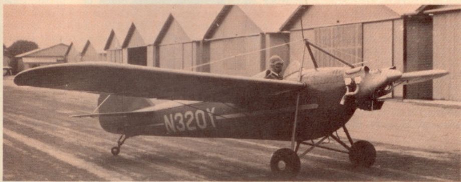
3. A modernized Pup with 65 h.p. Continental A65 engine replacing the original Szekely. Other improvements include steerable tailwheel and 8 by 4 wheels, with hydraulic brakes, from a Piper Cub. This one has pitot-static tube for air-speed indicator sticking out of the left wing.
