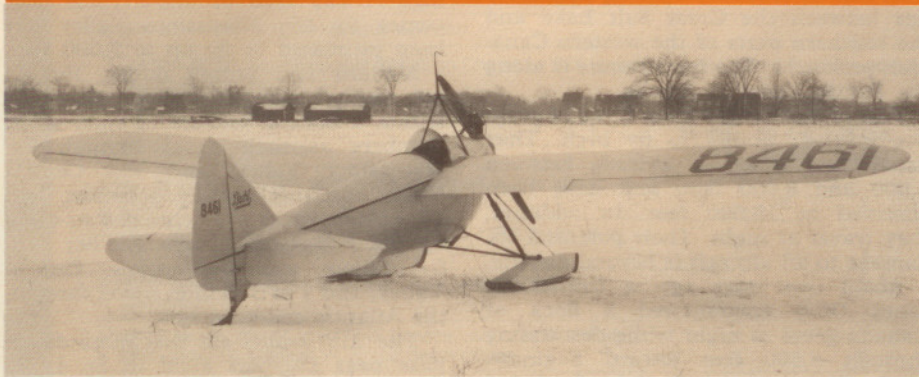
The little Buhl Flying Bull Pup was a versatile machine. This is the second prototype on skis. The use of a registration number alone, as shown here, means that the airplane is merely identified on government records and not yet licensed.
